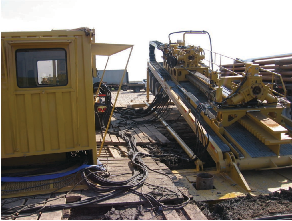
A modern fully hydraulic HDD drill rig with separate drill cab and power unit (hidden behind the drill cab).
