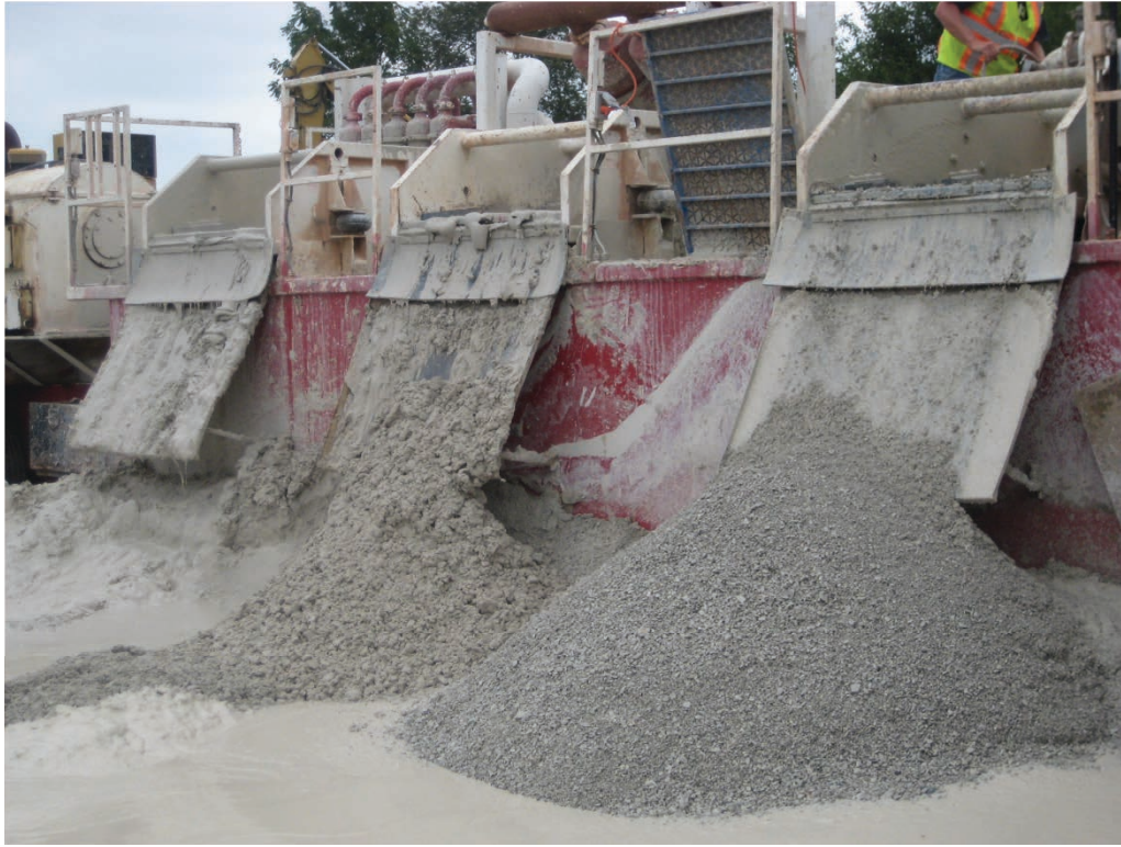
A three-stage drilling fluid recycling system.
