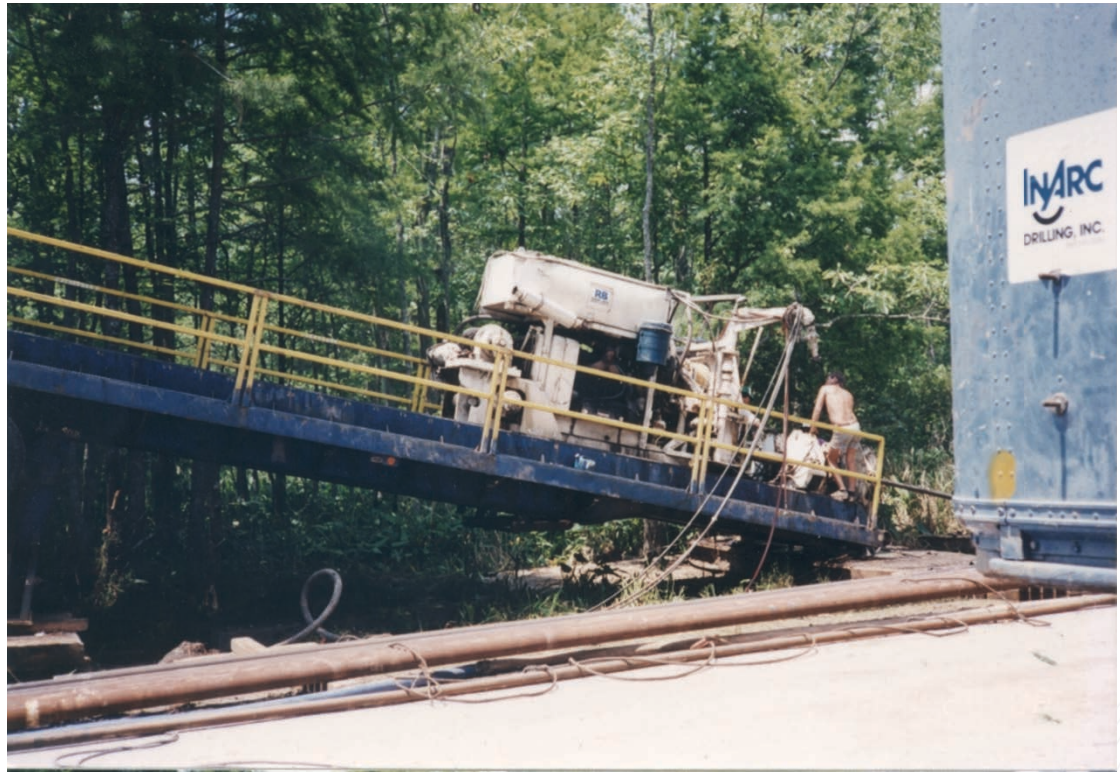
An early cable operated drill rig from from InArc Drilling
