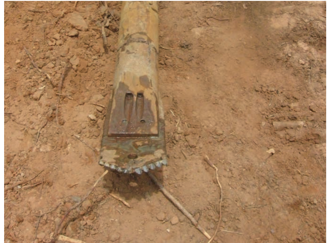
A duckbill style drill bit used for soil formations.
