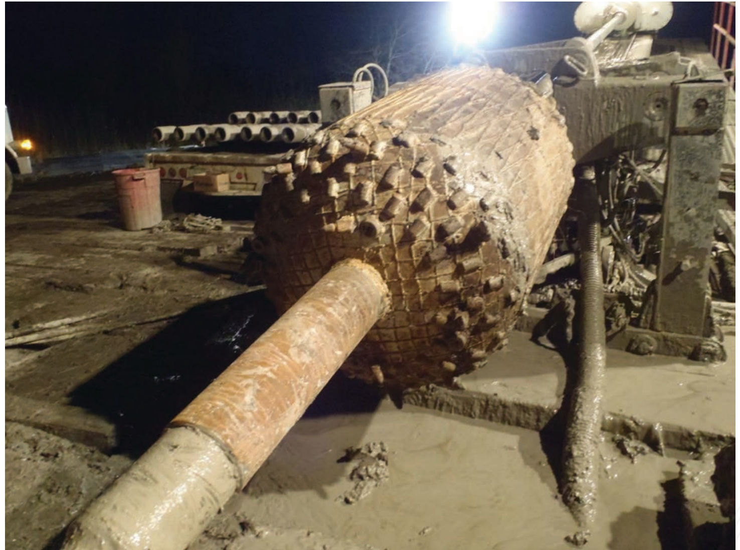
Barrel reamer used for swab passes.
