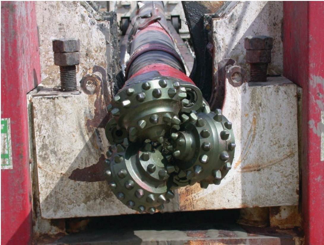
A tungsten carbide insert (TCI) tri-cone drill bit for medium hard rock formations.
