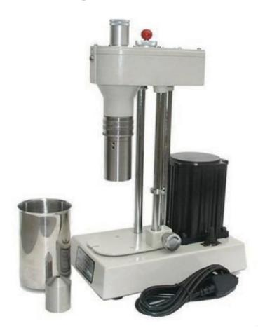
The rotational viscometer gives a more detailed measure of the condition of the drilling fluid. The resistance is calculated at 300 and 600 rpm and these values are used to calculate the PV and YP of the drilling fluid.
