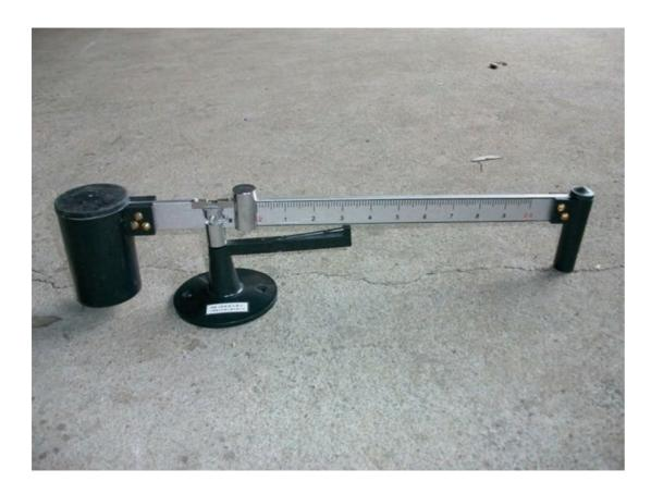
Mud balance scale. Used to calculate the drilling fluid unit weight.
