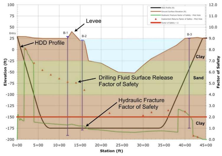
along the planned HDD profile to the anticipated drilling fluid pressure at that same point. The factors of safety against drilling fluid surface releases are shown at selected points shown as red triangles.
