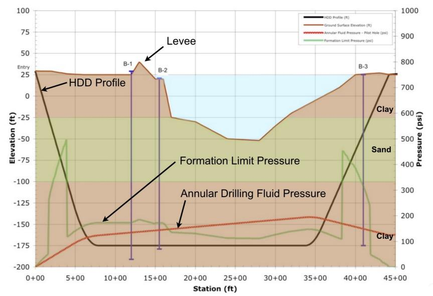
In the hydraulic fracture model, the formation limit pressure varies depending on the soil and bedrock encountered along the HDD profile shown as the green line. The estimated drilling fluid pressure is shown as the red line in and represents the estimated drilling fluid pressure along the HDD profile based on the anticipated drilling fluid properties.
