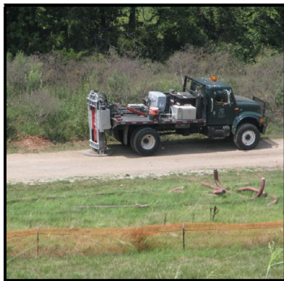
Photograph 4.1- Basin XLR8 Acoustic Source
