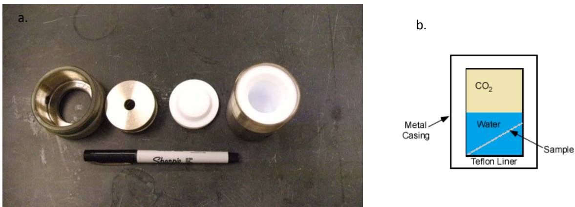
FIGURE 5.12. HIGH PRESSURE BOMB COMPONENTS. A) PHOTOGRAPH WITH THE TEFLON INSERT AND CAP VISIBLE AS THE WHITE COMPONENTS. B) SIMPLIFIED CROSS SECTION OF THE BOMB ILLUSTRATING SAMPLE PLACEMENT WITH RESPECT TO WATER AND CO 2 .
