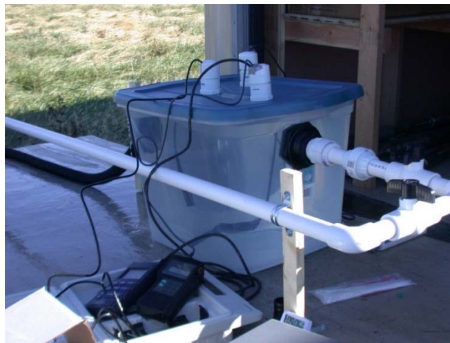
FIGURE 5.1. WATER BATH USED TO COLLECT WATER DIRECTLY FROM THE BOREHOLES. THE WHITE PVC PIPE REPRESENTS INFLOW FROM THE BOREHOLE AND THE BLACK EXIT TUBE IS SHOWN ON THE OPPOSITE SIDE. THE WHITE PVC CAPS ON THE TOP OF THE VESSEL HOLD IN-SITU MEASURING PROBES FOR PH, EH, TEMPERATURE, DISSOLVED OXYGEN AND CONDUCTIVITY. BLACK WIRES CONNECTING THE RESPECTIVE PROBES TO THE RECORDING INSTRUMENTS ARE VISIBLE LEADING FROM THE WHITE CAP POSITIONS.
